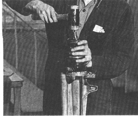
8.1 Drive the mainshaft home with a soft-faced mallet
