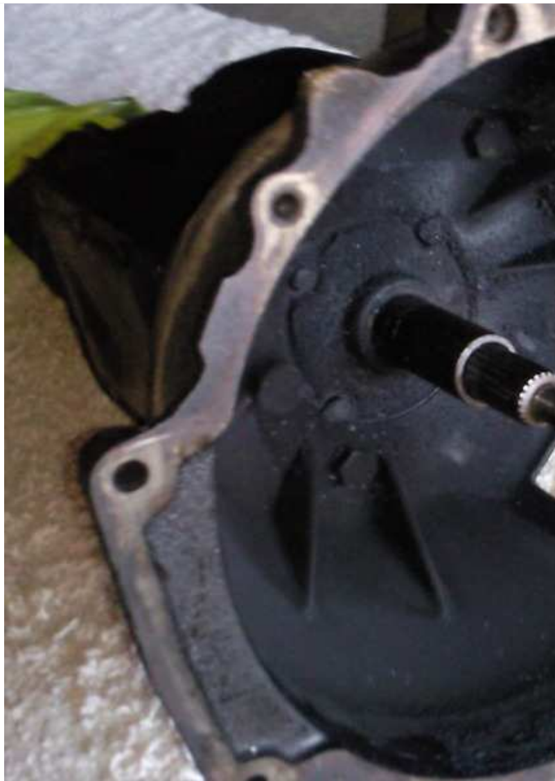
2.8 type 9 (longer input shaft)
