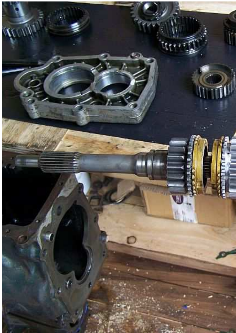
Layshaft cluster, (5th gear is missing in this pic, it goes on the end splines).
