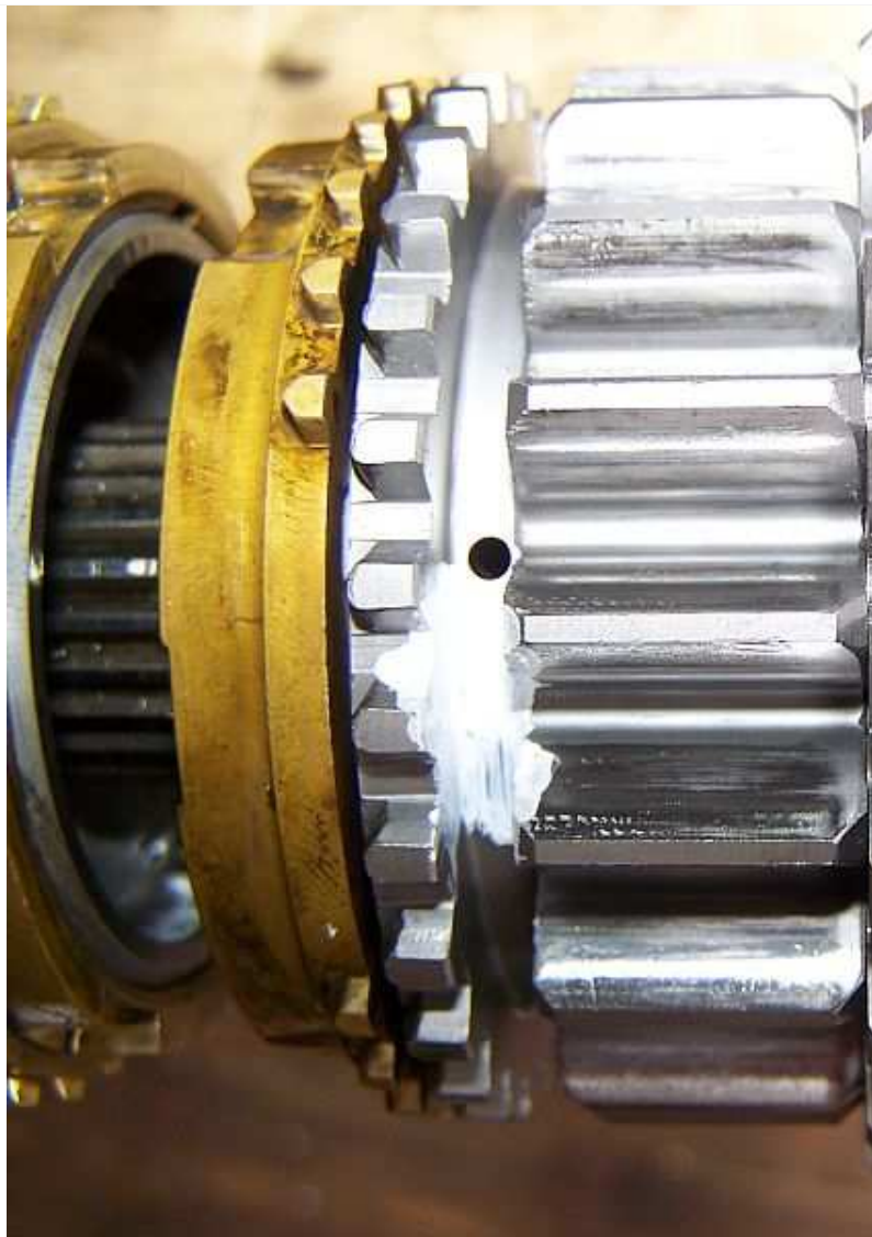
Bare mainshaft with gears removed
